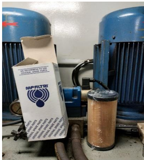
Fig.3. Changed Oil Filter Steering Gear
