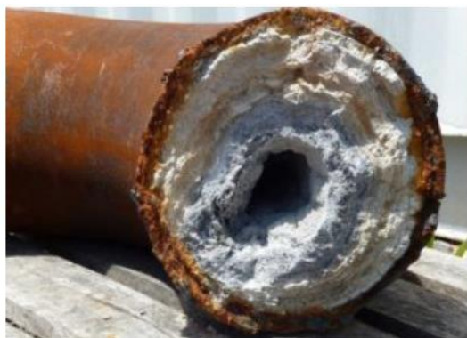
Figure 1. Silica scaling on geothermal pipes (Pusat Kajian Sumberdaya Bumi Non-Konvensional, FT UGM)
