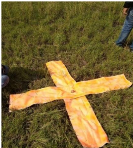
Figure 4. Installation of Premark.
