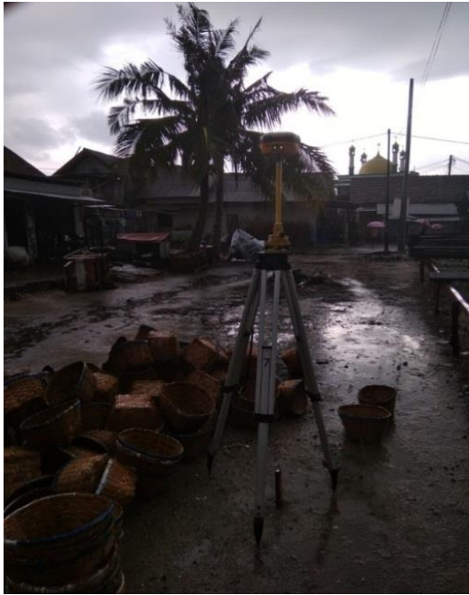
Figure 3. Ground Control Point Measurement.
