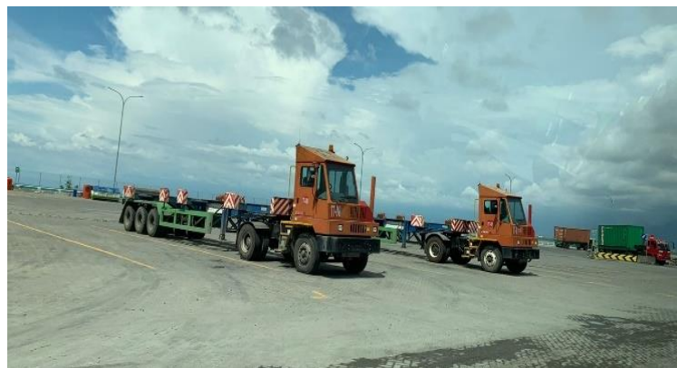
Figure 9 Eksisting Head Truck and Chassis Terminal II of the New Makassar Container Port
