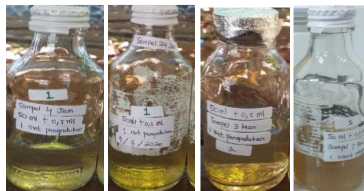
Figure 1. Solution of silver nanoparticles with different times (a). 4 hours; (b). 24 hours; (c). 3 days; (d). 7 days.
