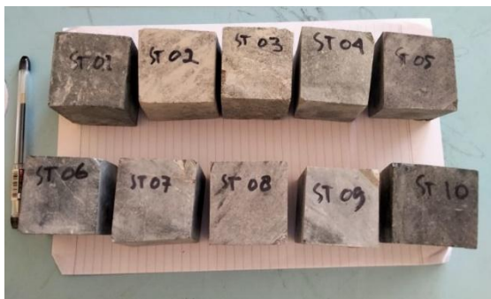
Figure 3. Rock example cut to size 4x4x4 cm.
